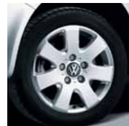
16" Miyato alloys 6.5J x 16 alloy wheels fitted with 215/65 R16 tyres.
